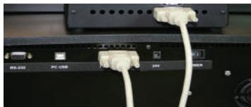
**Figure 114. Cable connection of injector system to GloMax<sup>®</sup> Discover Instrument.**
