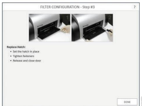
**Figure 87. Replacing the hatch door.**
