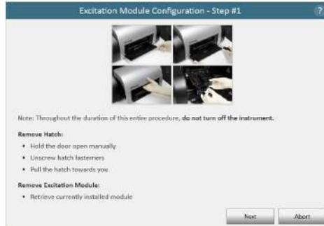
**Figure 88. Custom Fluorescence Excitation Module configuration procedure.**
