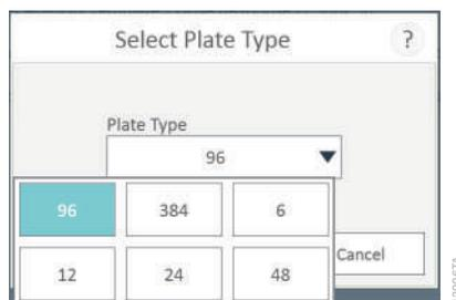
**Figure 61. The ‘Select Plate Type’ screen.** When creating a new analysis template, the first step is to select the plate format for the analysis template from the drop-down list on the ‘Select Plate Type’ screen.
