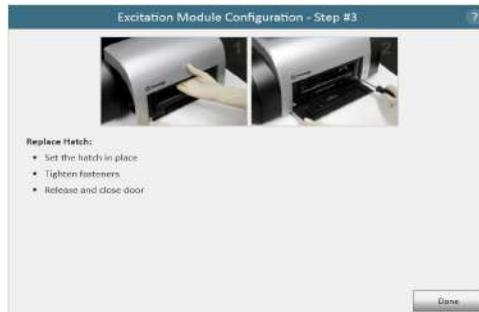
**Figure 90. Replacing the hatch door.**
