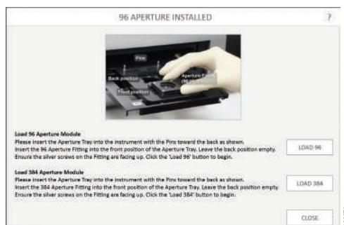
**Figure 91. Aperture loading instructions screen.**
