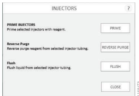
**Figure 115. Injector functions (prime, reverse purge and flush).**
