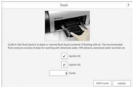
**Figure 118. Injector Flush function.**
